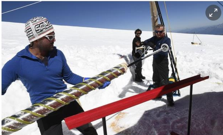
Members of the "Protecting Ice Memory" project extract an ice core piece out of a drill machine in their camp at the Col du Dôme. Photograph: Philippe Desmazes/AFP/Getty Images
